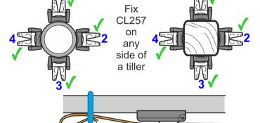
**KElastic** When Mounting in positions 2,3 & 4 use an elastic band to hold the tail of the rope.
